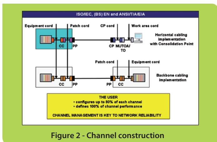
Figure 2 - Channel construction
