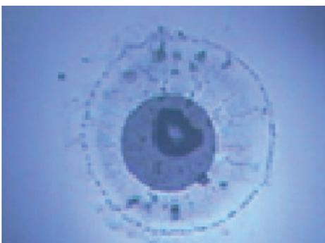
Even the use of 'dirty' dust caps can have a significant impact on the 'cleanliness' of the fibre installation. The oil from human skin can also have a dramatic effect when viewed under a microscope.
